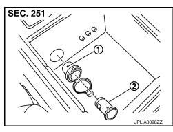
CONSOLE POWER SOCKET: Removal and Installation
